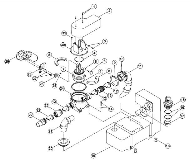
**NOTE**: When reassembling pump, tighten screw (Item No. 31) , to 20  $\pm$ 2 lbs., or until snug. Overtightening will cause holes to strip.
